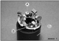
• Remove the nut and terminal bolt [A], and then remove the brush [B] and the plastic holder [C].
