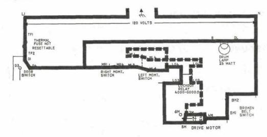
When the motor centrifugal switch opens, the circuit which was bypassing the relay coil, is no longer complete. Current must now flow through the lockout relay coil. The energized relay coil opens the relay switch, opening the circuit through the motor run winding.
