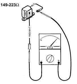
2. If meter readings are other than specified, replace trigger coil. Refer to "Ignition Components Removal and Installation," following.
