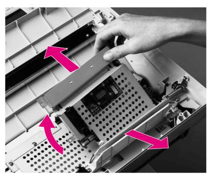
Figure 81. Remove the scanner controller
