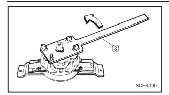
• Tighten the spider to specification using the bar wrench ③.
